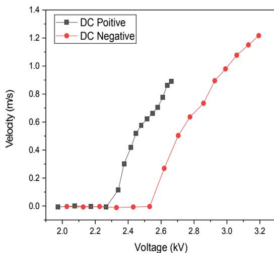
**Figure 8: Velocity is plotted with respect to applied voltage between the wire (Pt, d ¼ 25 µm) and ground electrode (D ¼ 4 mm).**
