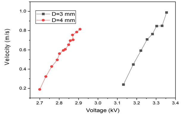
Figure 5: Velocity is measured with respect to electrical power
